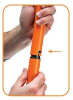
Turn the lower tool body clockwise to lock it into place.
